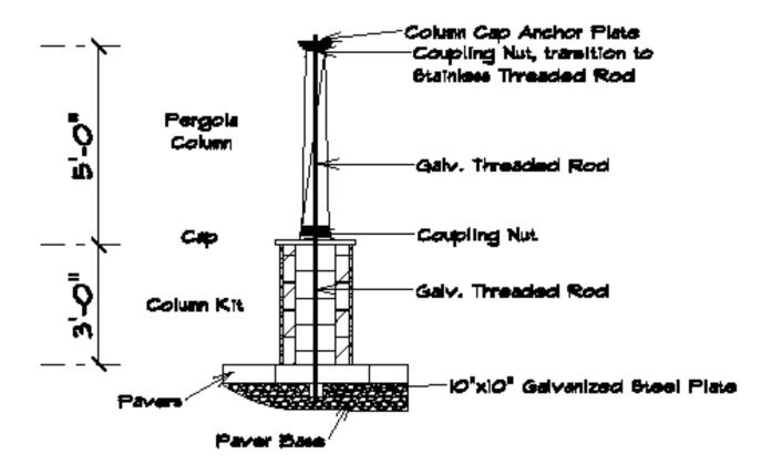
Insert threaded rod into steel bottom plate and attach second rod using coupling nut. Position the four plate and rod assemblies as per the footing layout.
