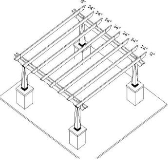
Align rafters with the spacers between the Beam Assembly. Secure by putting 9 inch wood screw through pre drilled hole in bottom of spacer, and into the rafter above.
