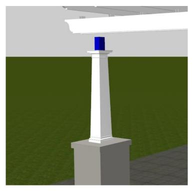
Seat Beam Assembly over Column Assembly and attach using aluminum bracket
