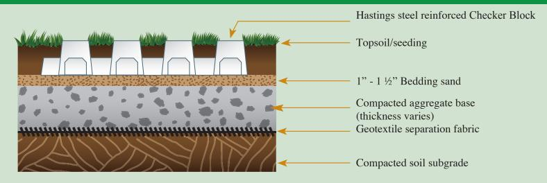
Checker Block is a unique castellated concrete grid paver ideal for heavy duty applications that require full turf establishment. The product is used for commercial and residential applications such as emergency access, fire lane, service roads, parking lots and pathways. It is also ideal for erosion control to stabilize embankments, stream ways and swales. Some of the key advantages of Checker Block include:
