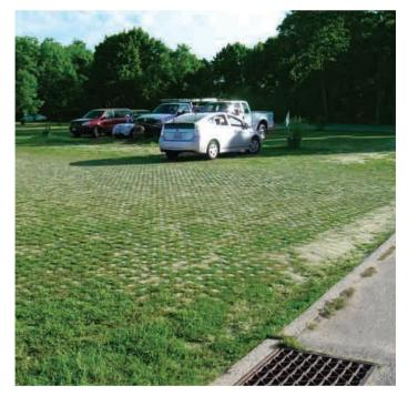
"Checker Block is a Low Impact Development solution for parking when a grass lawn is desired", said Matt Rocchio, General Manager for Sands Point Preserve . "The pervious and durable nature of Checker Block allowed us to avoid traditional impervious blacktop or concrete pavement which would have increased stormwater runoff to the Long Island Sound and tarnished the stately appearance," he added.
