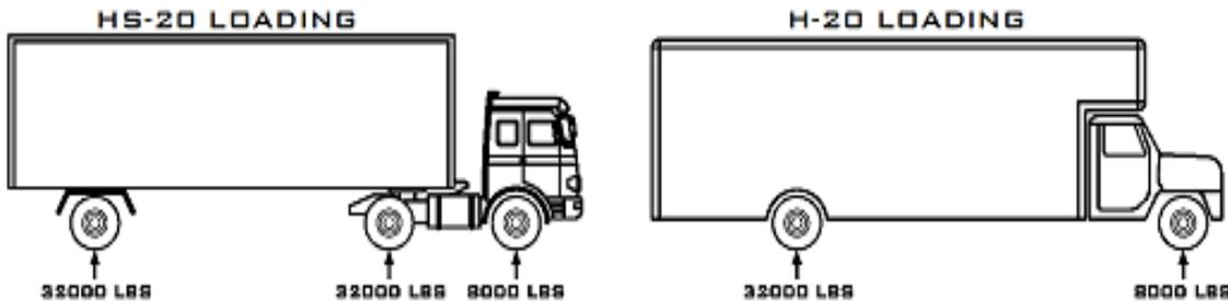
**Step #1) Determine the maximum wheel load:**
